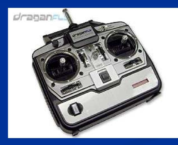
The transmitter communicates your stick positions, via a radio signal, to the RC model airplane. The RC model airplane contains a <u>receiver</u>, which decodes this transmission and tells the <u>servos</u> to move a position corresponding to what you commanded on the sticks. The servos are a cool piece of technology. They rotate to whatever position they are told to go to, and are very strong and very accurate.
